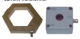
When a current transformer is used instead of a quadrupole, the current transformer can be placed around a coupling capacitor terminal or around a part of the test object itself. A current transformer has the advantage of providing galvanic isolation between the PD detector and the high voltage circuit. Current transformers are offered as separate modules or integrated with a coupling capacitor into a single unit.
